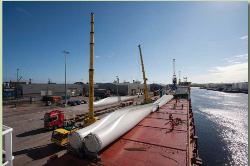
Offloading blades at Aberdeen Harbour destined for RES' Hill of Towie Wind Farm, Scotland.
