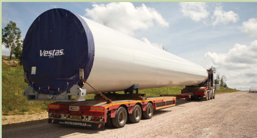
Tower section being transported to turbine location on site at Wadlow Wind Farm, Cambridgeshire. Photo courtesy of BIF.
